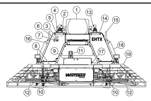
Figure 2. EHTX Controls and Components (Front)
